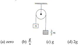
26. In the figure given below, with what acceleration does the block of mass *m* will move ? (Pulley and strings are massless and frictionless)
